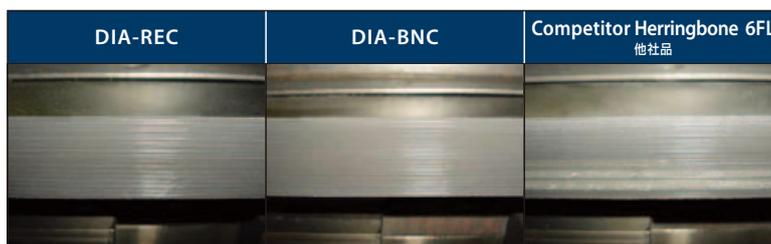
By reducing the cutting force, stable milling even under low rigidity is achieved.
