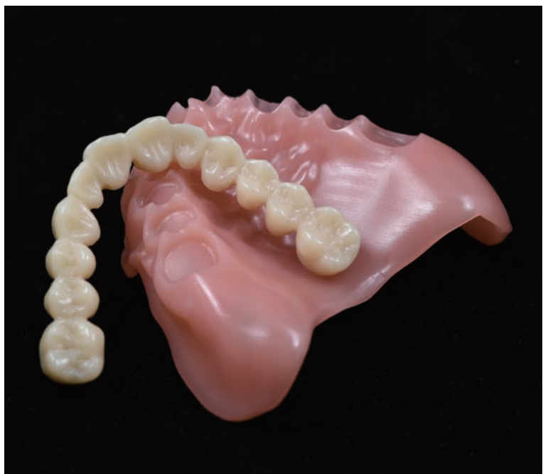
Milling is performed using micro tools from OSG. To achieve the high precision required for components such as cores or prostheses, re-milling is conducted in 2-micron increments. Photo courtesy of ZM Solutions AG.
