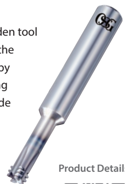
Figure 7. AT-2 carbide thread mill with end-cutting edge for high-hardness steels. By performing helical drilling and threading simultaneously, the consolidation of machining process in highly difficult high-hardness steel applications is made possible.
