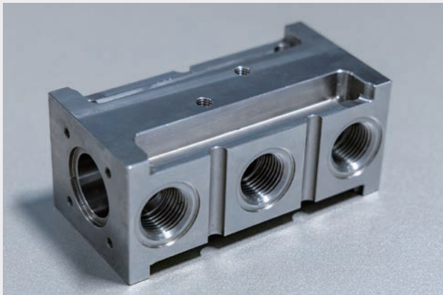
A hydraulic distributor made of 316L stainless steel, a key component in hydraulic systems. Each hydraulic distributor requires the drilling of 12 blind holes in two sizes and five through holes at a diameter of 13 mm.
