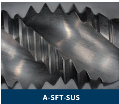
■1,000穴加工後 Cutting edge after tapping 1,000 holes
