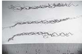
新仕様品で加工の切りくず Chip from new specification product
