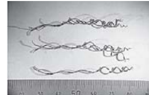
従来仕様品で加工の切りくず Chip from old specification product
