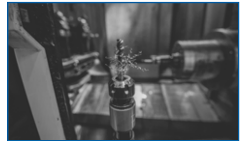
From left, OSG Sales Technician Valdir Lima and Valtra Applications Engineer Jeferson Barreto inspect the condition of the XPF forming tap used for threading fuel tanks in SAE 1020 steel.
