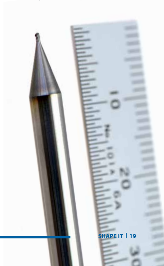
Thanks to its unique 3-flute geometry, the PHX-LN-DBT can serve as a finishing tool. Further, the PHX-LN-DBT's strong helix angle ensures that the tool exhibits very low radial deviation to accommodate tight tolerance requirement.
