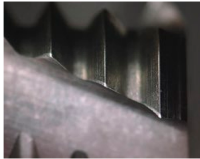
1本目 8,800穴加工後 No.1 (after cutting 8,800 threads)
