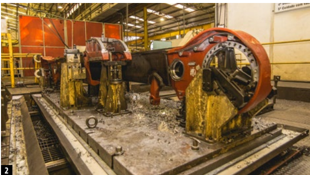
2 A track frame, which is a side-frame component of the bulldozer, waits for completion at Komatsu do Brasil's production plant in Suzano, São Paulo.
