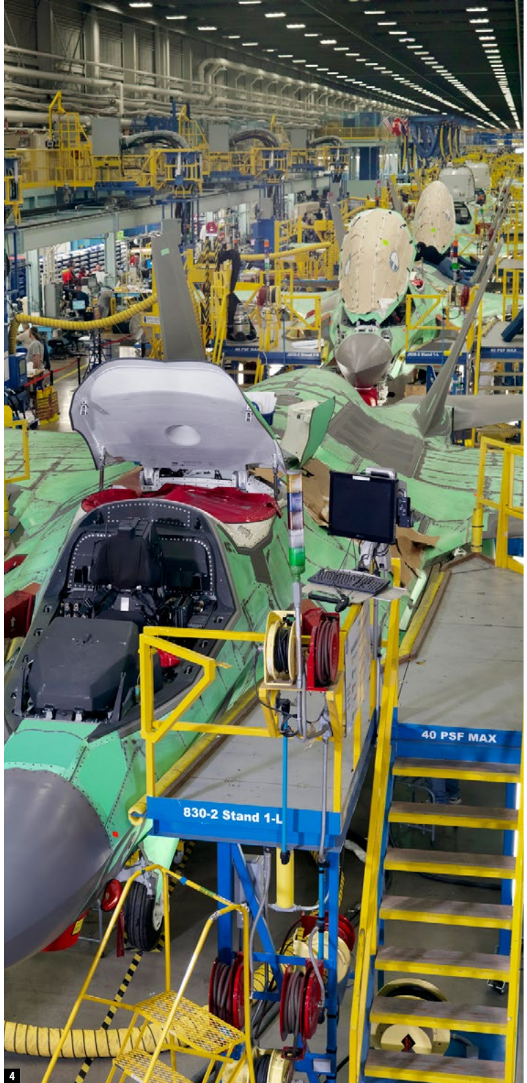
4. F-35 production line in Texas, USA. With capabilities to eliminate delamination in the routing of advanced carbon fiber (CFRP) composite wing skin material while achieving significantly longer tool life versus other cutting tool providers, several AMAMCO diamond-coated tools are currently used by Lockheed in drilling applications on the F-35. Photo courtesy of Lockheed.
