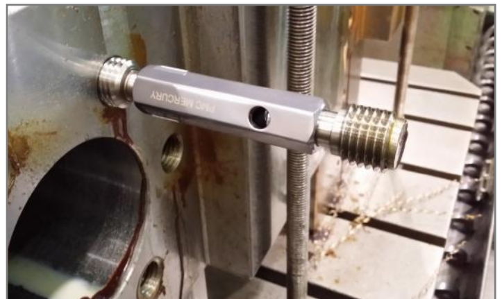
FMC's very own 1" 8UNC GO plug gauge was used to confirm the accuracy and finish of the thread surface. The thread tapped by the A-SFT appears in good quality.
