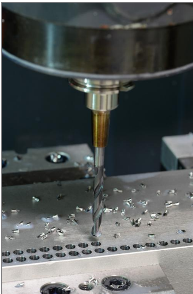
Lower cutting force and less friction for reduced cutting temperature and a new chamfer design for lower feed rates and optimal chip formation are proven results achieved by OSG with the WDO-SUS coolant-through carbide drill series.
