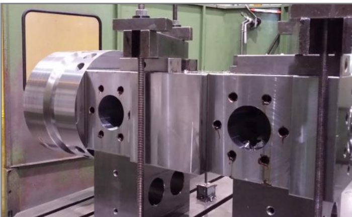
An annulus block valve in a R16-3100 machine at FMC Technologies.
