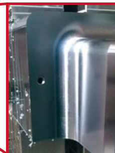
1ワーク88m(3時間)加工後の刃先の損傷状態 Cutting edge after 88m (3 hours) of milling
